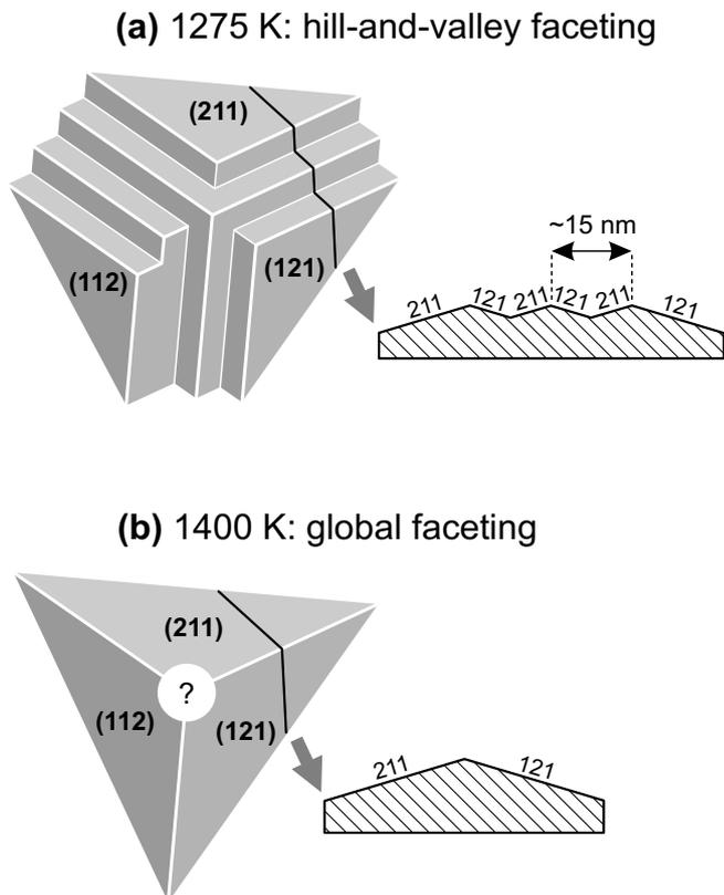
FIG. 2: A simplified model of the crystal topography in the vicinity of the  $\langle 111 \rangle$  pole. The crystal cross-sections shown on the right run along the  $\langle 113 \rangle$  plane (perpendicular to the facet edges). The detailed shape of the vertex region in (b) could not be determined in this experiment.
