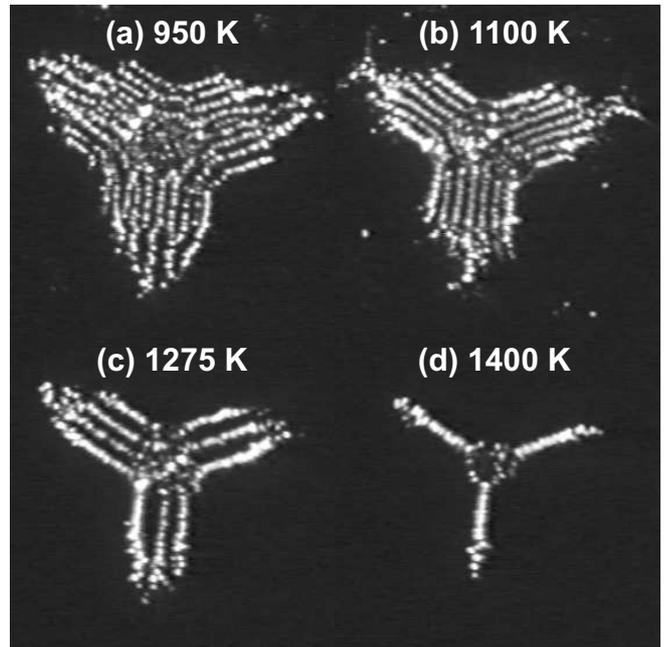
FIG. 3: Microscopic images of the crystal surface in the vicinity of the  $\langle 111 \rangle$  pole. Edges of the facets are imaged as bright lines. The interpretation of these images is proposed in Fig. 2.
