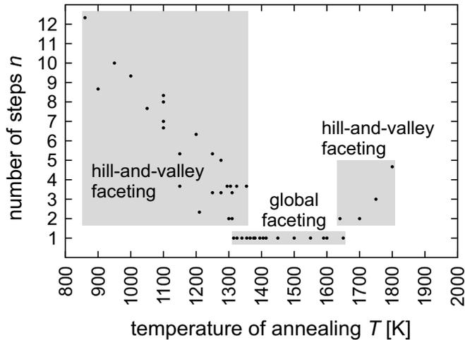
FIG. 1: Number of  $\{211\}$  steps in the vicinity of the  $\langle 111 \rangle$  pole. If  $n = 1$ , a single  $(211)$ - $(121)$ - $(112)$  pyramid is formed (global faceting).
